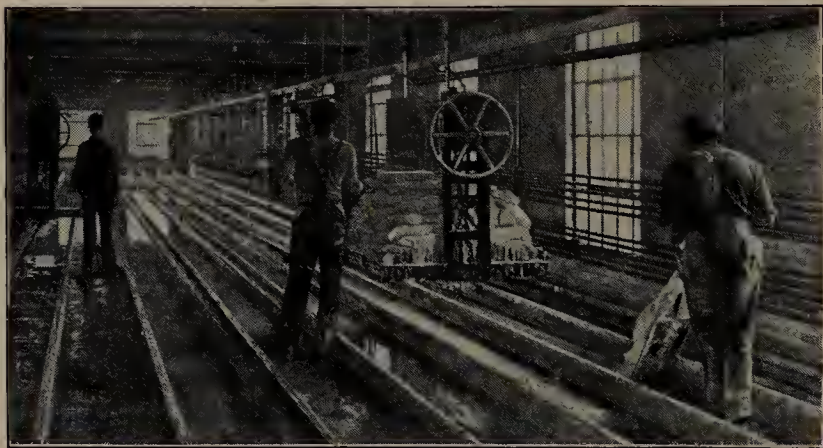
FIG. 130. Removing the starch from the settling troughs in a starch factory
